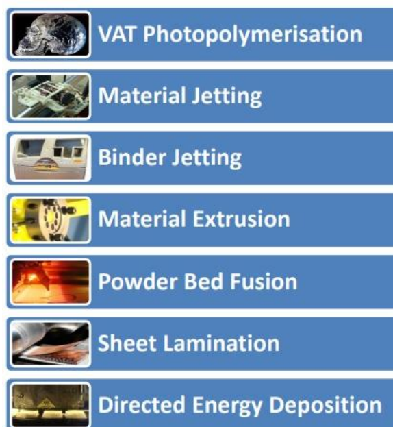
Figure 9: Additive manufacturing methods based on [32]
