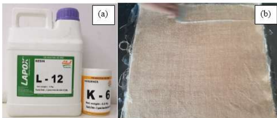
Fig.1: (a) Lapox L 12-Resin and K-6 Hardener (b) Fabrication of hybrid composite using Hand Layup Technique.
