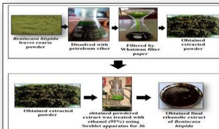
Fig 2: Extraction Procedure by using soxhelet apparatus
