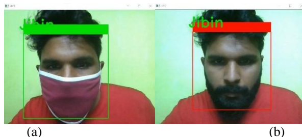
Figure 14 Combined model: Face recognition and mask detection (a)with mask (Person's biometric in a green bounding box) (b)without mask(Person's biometric in a red bounding box)
