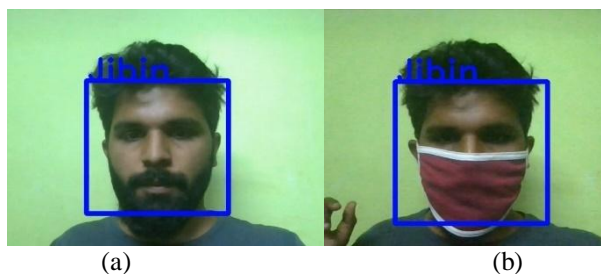
Figure 13: Face Recognition Using LPBH algorithm (a) Face recognition of the person (b) Face recognition with mask
