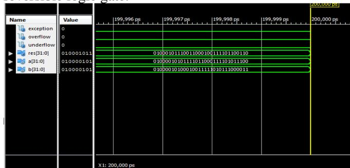
**Figure.17:** output waveform of reversible logic for FP multiplier
