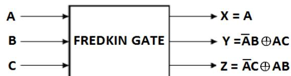
A block diagram of a  $3 \times 3$  Fredkin gate is shown in figure 5
