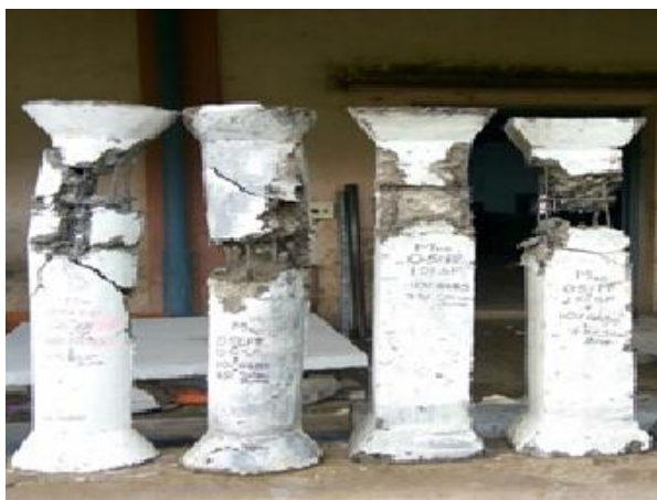
Fig.13 Failure of M70 GPC model specimens without fibers Fig.14 Failure of M70 GPC model specimens with fibers
