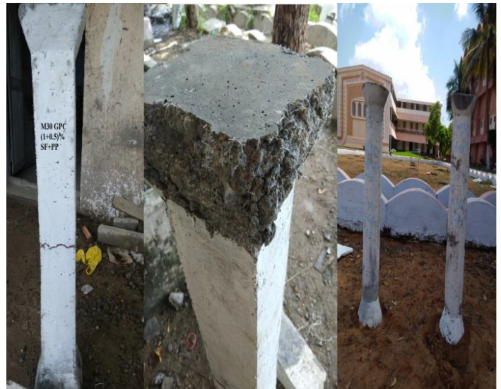
Fig.11 Failure of M30 GPC model specimens without fibers Fig.12 Failure of M30 GPC model specimens with hybrid fibers
