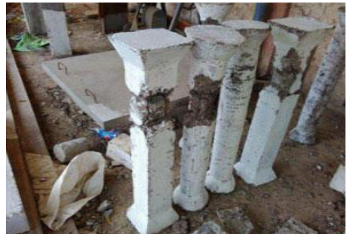
Fig.13 Failure of M70 GPC model specimens without fibers Fig.14 Failure of M70 GPC model specimens with fibers
