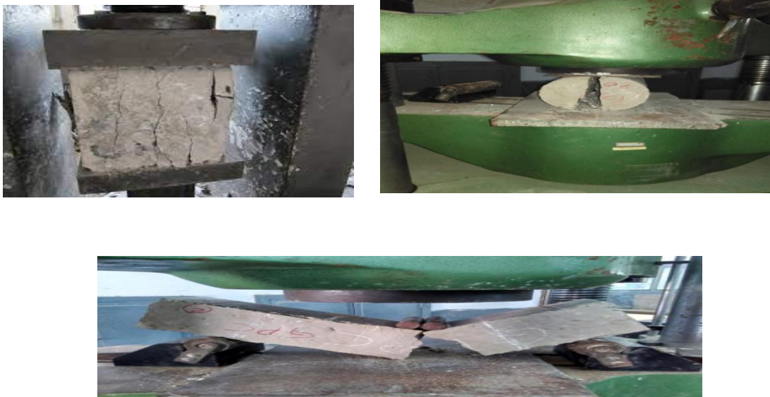
Fig.2 Specimens under Compression, Split-tensile and Flexural Strength Tests
