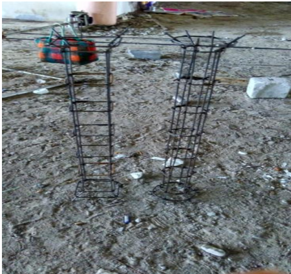
Fig.9 Square and Circular Head Reinforcement Cages Fig.10 Test Setup Arrangement
