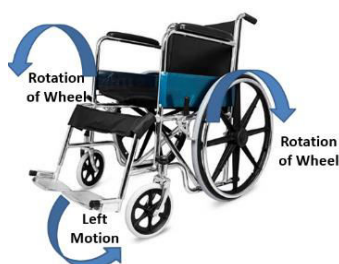
Fig.5 – Left hand gesture and motion of wheelchair in left direction
