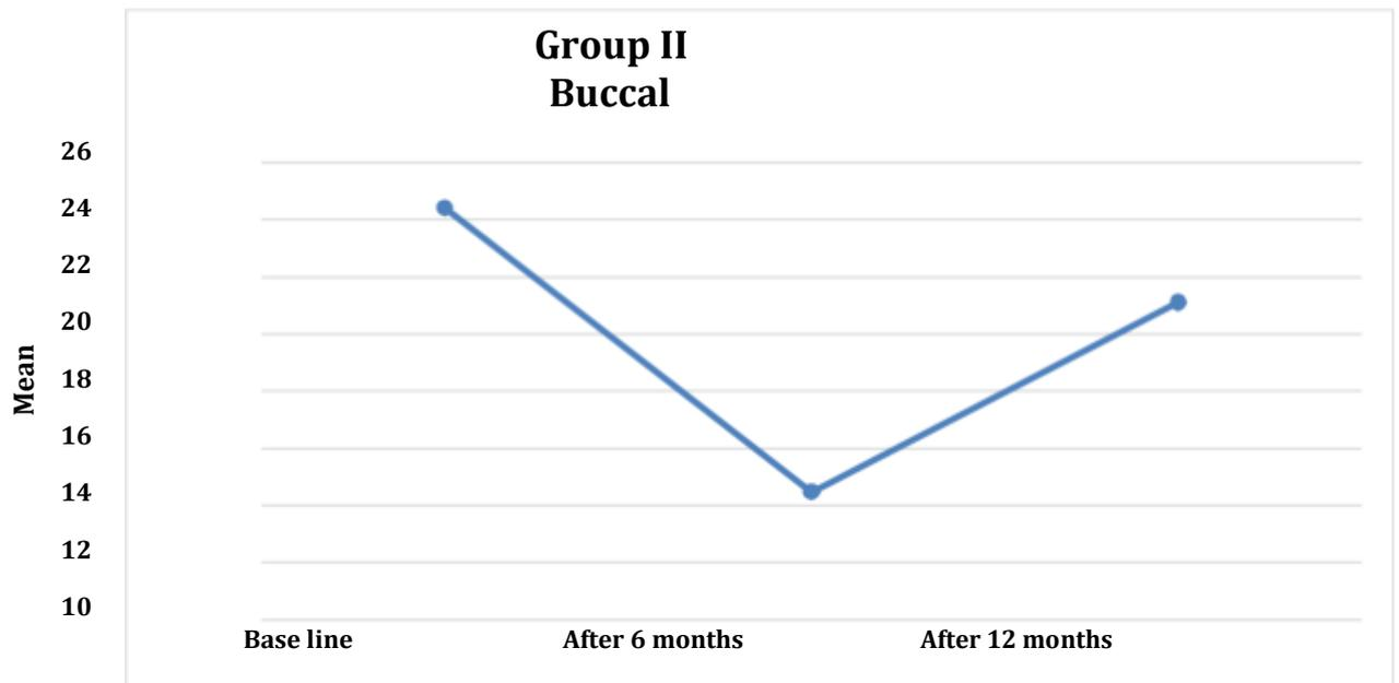
**Figure 16:** Line chart representing retention of group II; baseline, 75,000cycles (equivalent to 6 months) and 150,000cycle (equivalent to 12 months)
