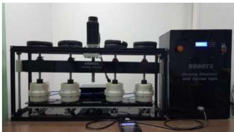
**Figure 15: Represent chewing simulator machine (Robota)**
