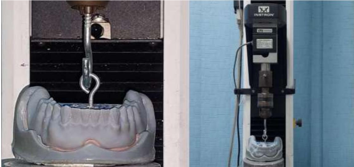
**Figure 14: demonstrate the universal testing machine attached to the model**
