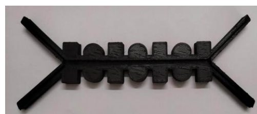
Figure 6: 3D printing of the designed channel using Polylactic Acid (PLA)
