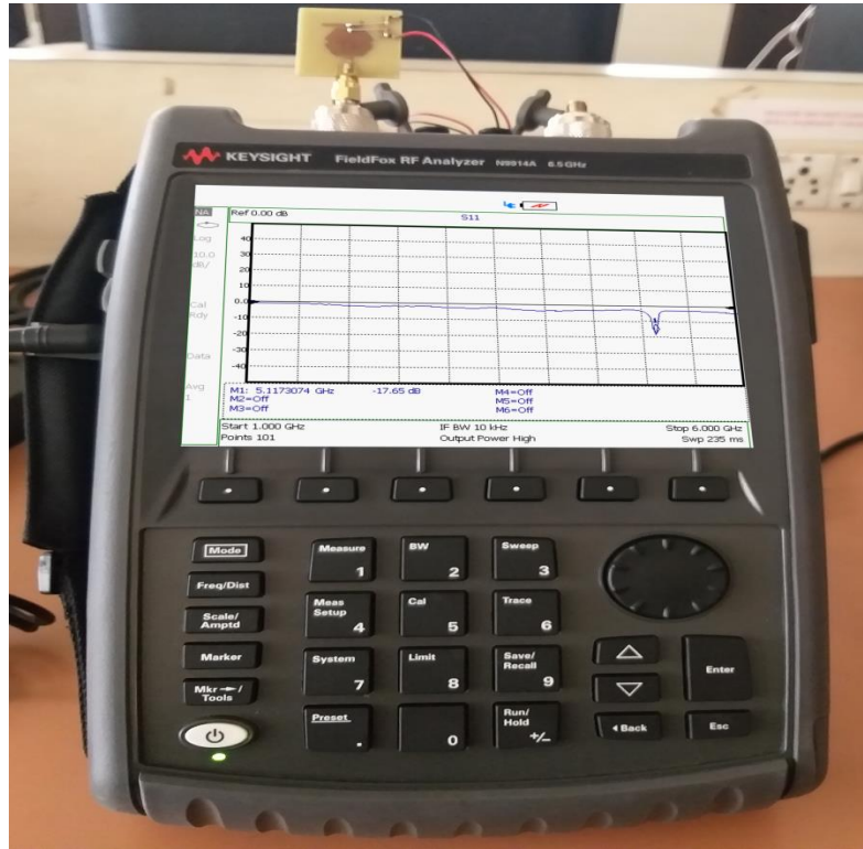
Figure 12: Analyser set up for Antenna testing
