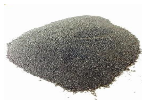
Figure 3. The physical shape of nickel slag as a fine aggregate
