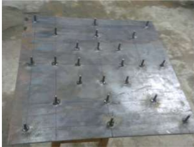
Figure 3 Steel plate with shear studs (S-5) [4]
