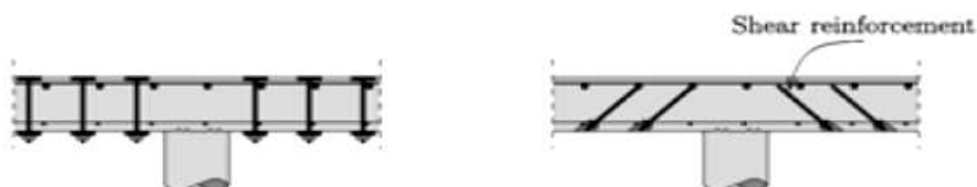
Figure 6. Usual applicable solutions for strengthening of deficient flat slabs against punching (Fernandez Ruiz, 2011) [11]
