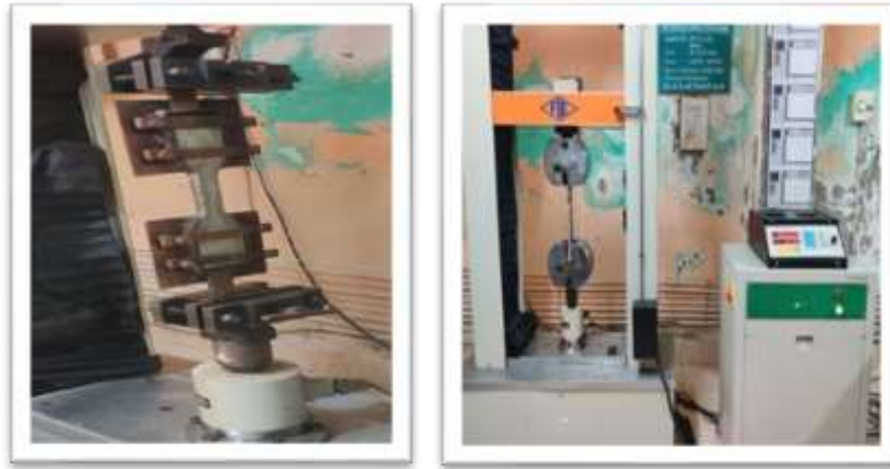
Fig 9. Direct tension Testing Setup
