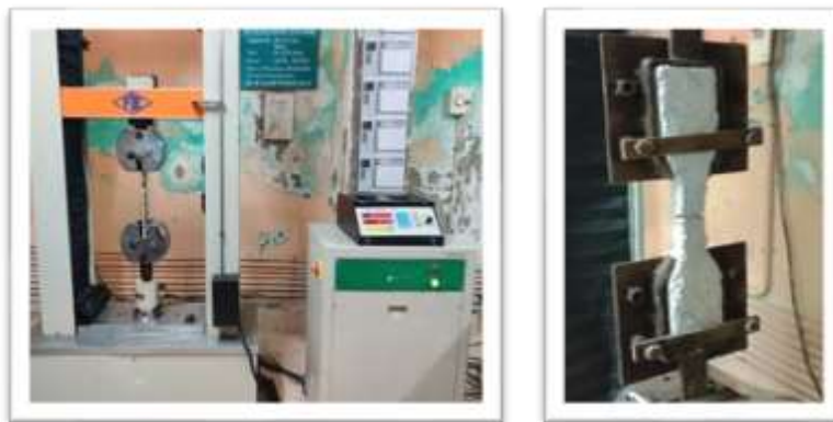
Fig 11. Direct Tension test on Notched Dog bone Specimens
