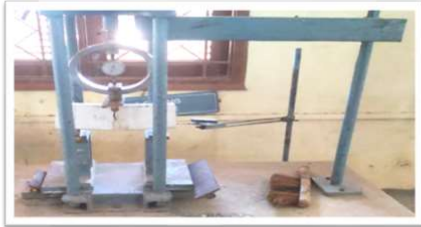
Fig 10. Three Point Bending Test setup
