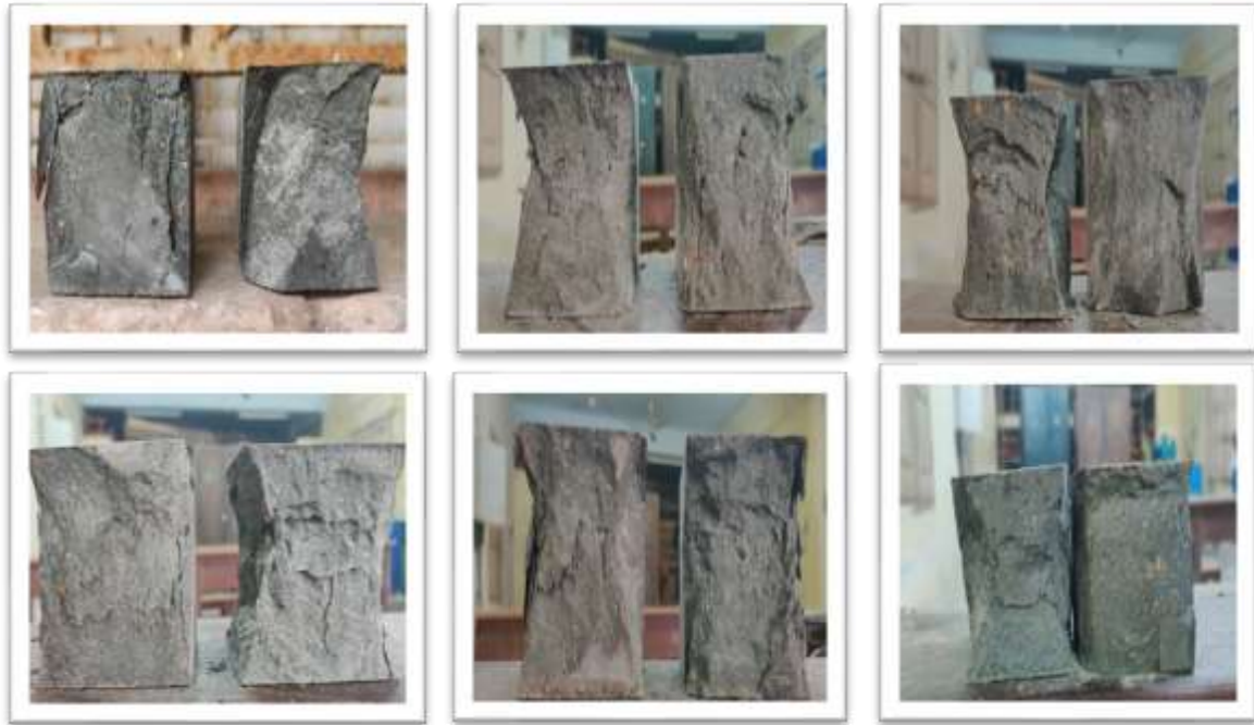
Fig 13. Failure modes of the mortar cubes
