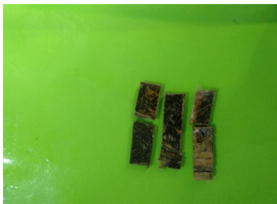
[Fig 7. Specimen after charpy test]
