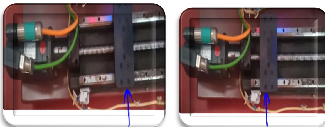
Fig. 3. (a) Position reached by the Lead Screw from Start Position (0 LU) to Relative Position (200 LU) (blue arrow) Home Position reached by the Lead Screw (blue arrow)
