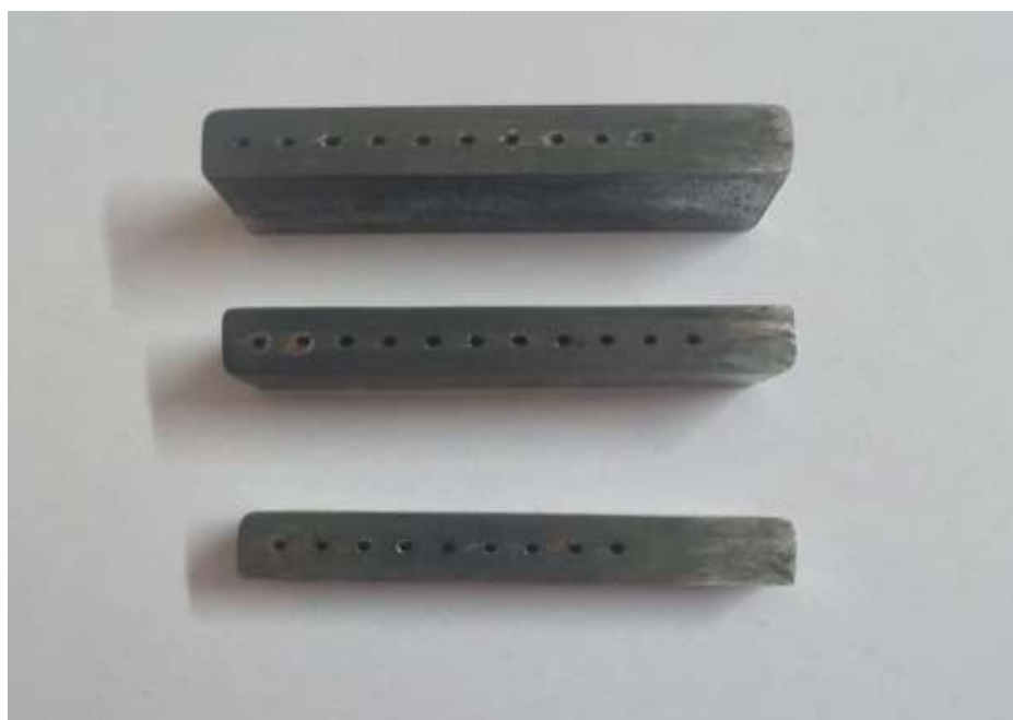
Figure 2. Meso holes Produced on EN_31 Steel by Electrical Discharge Drilling with 10mm, 15mm, 20mm thickness
