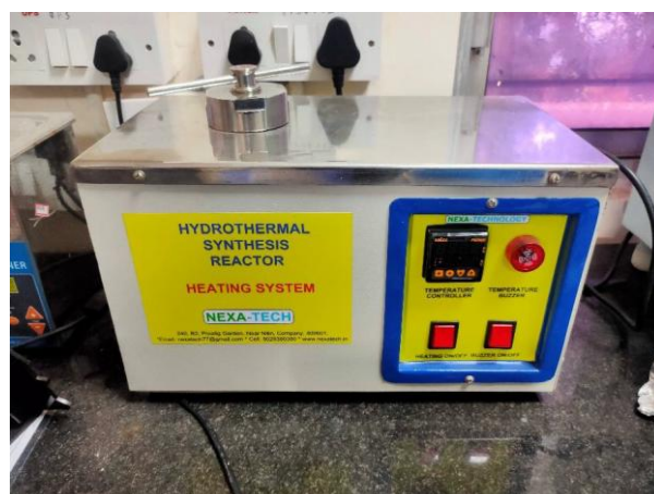
Figure 2: Hydrothermal Synthesis Reactor
