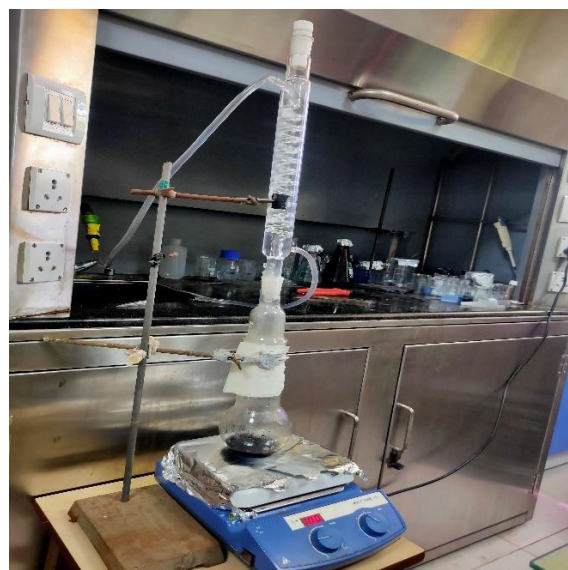
Figure 1: Acid Treatment using Reflux Set-up
