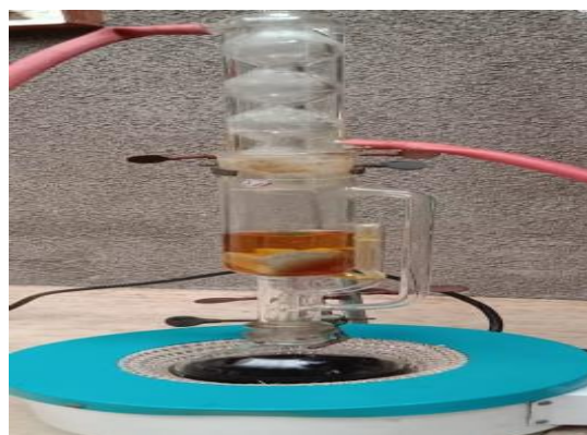
Figure 2: Preparation of Plant extract in Soxhlet apparatus
