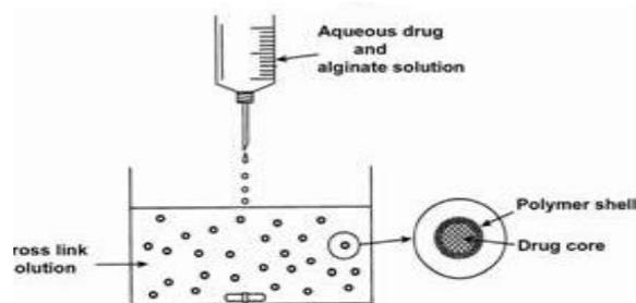
**Figure -3** Procedure of microsphere preparation of ionic gelation method
