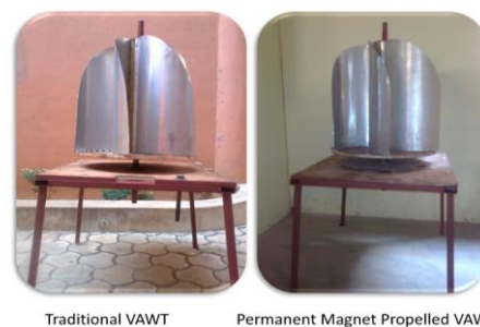
Figure 1: Savonius type modified turbine.
