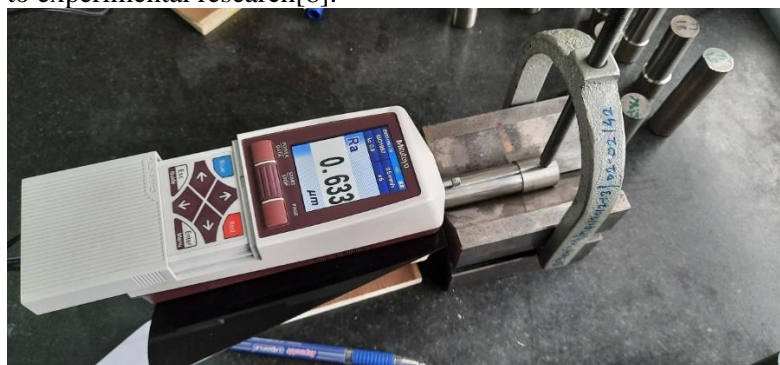
Figure 1 Roughness measurement by Ra (surface roughness) Tester
