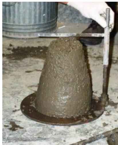
Fig: 2. Measuring Slump Fall
