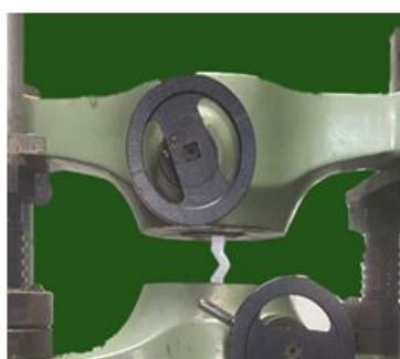
Figure no 8: Trouser shaped specimens in universal testing machine for checking tear strength
