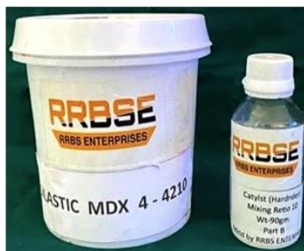
Figure no 5: Silastic 4- 4210 Elastomer (base and catalyst)
