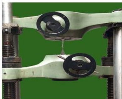
Figure no 9: Dumbbell shaped specimens in universal testing machine to check percentage elongation
