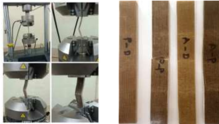
Fig-2 compression test of the specimens Fig-2.1 specimens after Compression Test
