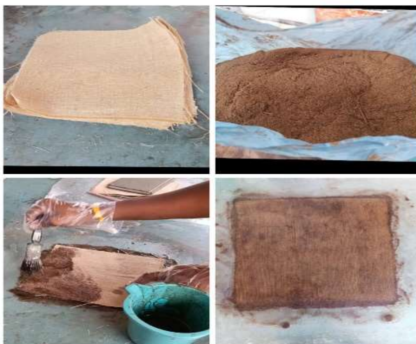
Fig-1 Preparation of laminates by using Araldite L556, Polyester, and Areca trunk husk
