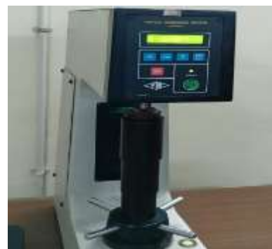
Fig-5.1 Hardness Test using Rockwell Machine
