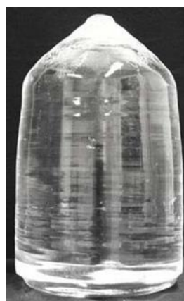
Fig. 4. Czochralski method for growing CaF 2 crystal with 200 mm diameter. [12]
