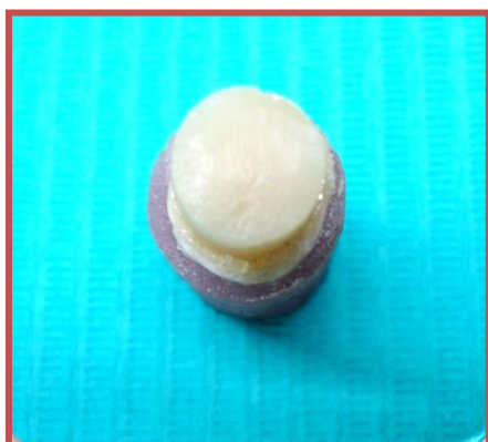
Figure (11): The acrylic block with the bonded composite resin
