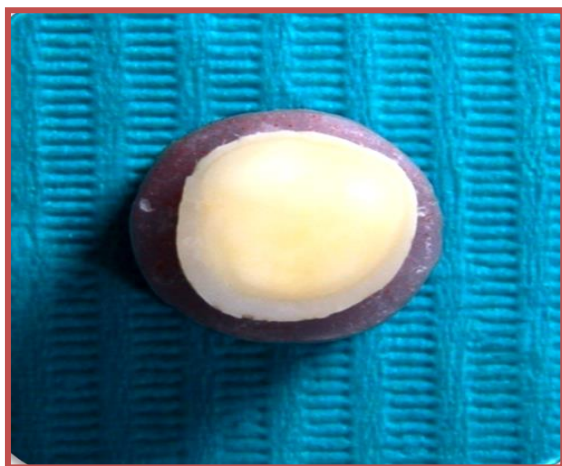
Figure (9): The prepared tooth specimen embedded in the acrylic block
