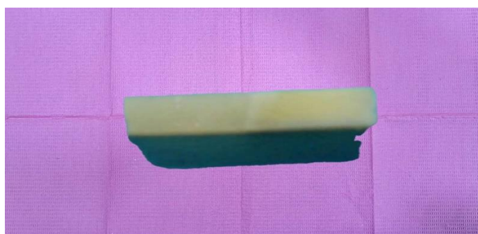
Figure(13): A beam consisting of a composite, bonding agent and dentin parts.
