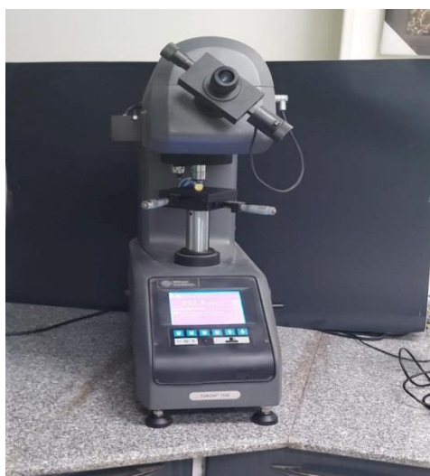
Figure (21): Depth of curing test by Vickers microhardness test.
