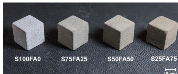
Figure 4.3 3D printed green cubes using geopolymer powder with different slag/fly ash ratio
