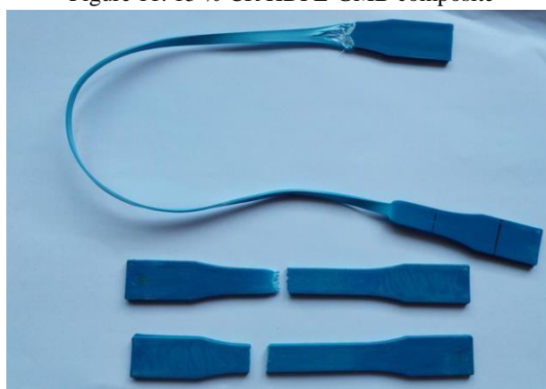
Figure 12. 5%, 10%, 15% CR Composite After Tensile Test
