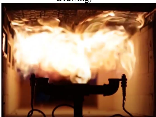
Figure 26: specimen in the ceiling position with the surface to be evaluated exposed face down to the ignition source. (Crimi, 2018)
