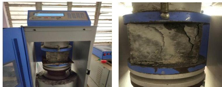
Fig.2. Compression Testing of Control Mix at CTM
