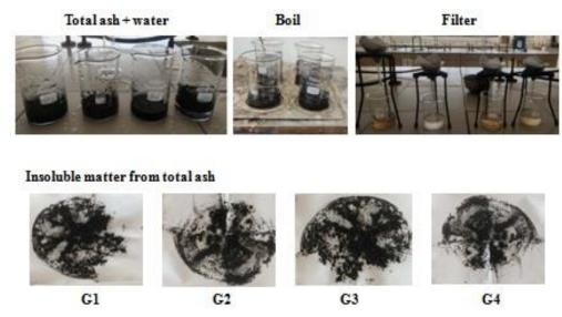
Fig. 9 water soluble ash value detection
