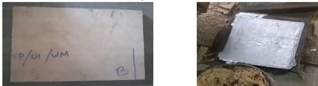
Figure 3. Solidified AlTiO 2 after casting Figure 4. AlTiO 2 work piece after forging process
