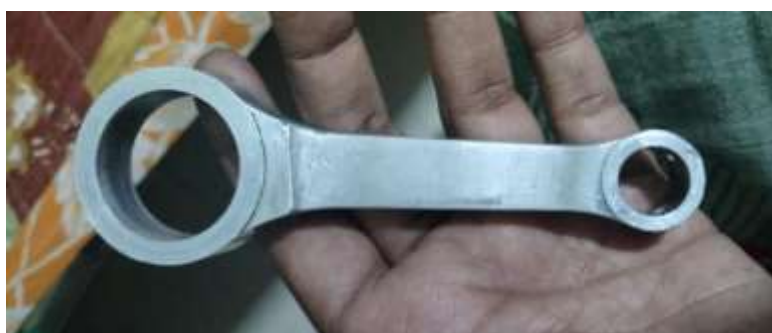
Figure 11. Condition of AlTiO 2 connecting rod after test performance
