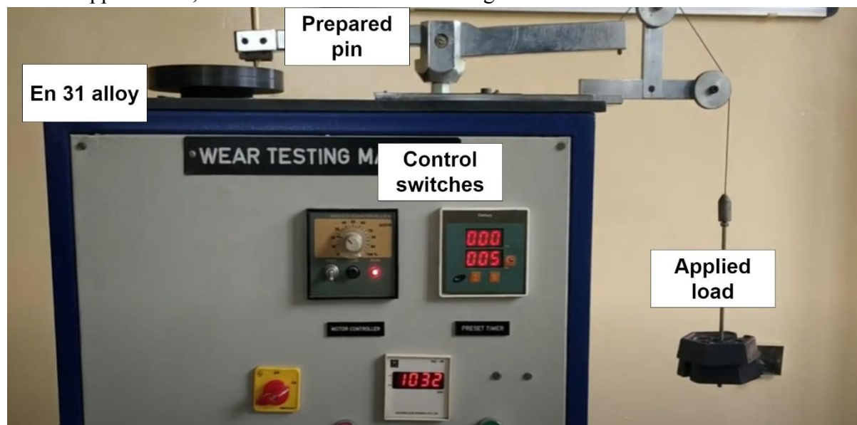
Fig. 2. Pin on Disc wear test apparatus
