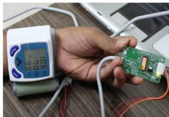
Fig. 4 : Patient's data collection using Blood pressure Sensor
