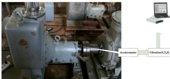
Figure 2: centrifugal pump setup for data acquisition
