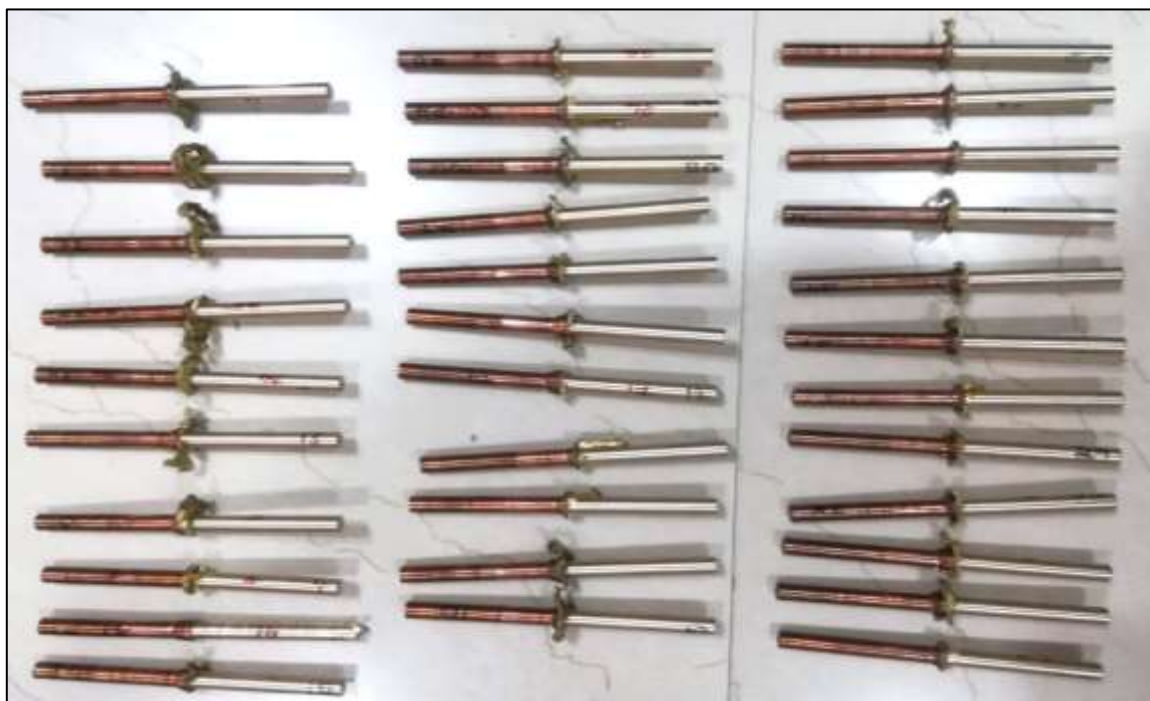
Figure 13. Joints after FW
